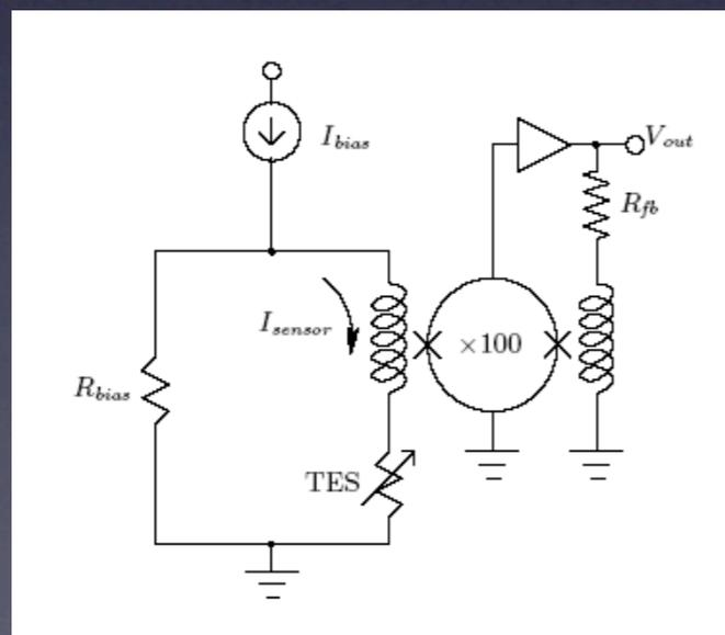
Electro-thermal feedback schematic
