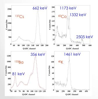
**High energy**: external sources of gamma rays (e.g. <sup>137</sup>Cs, <sup>60</sup>Co and <sup>133</sup>Ba) and gamma rays of 1461 keV due to <sup>40</sup>K decays in an adjacent detector, tagged by the 3.2 keV X-rays
