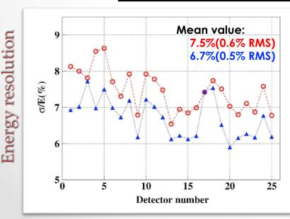
$\sigma/E @ 59.5 \text{ keV for}$ each detector with new PMTs with higher quantum efficiency (blu points) and with previous PMT EMI-Electron Tube (red points).
