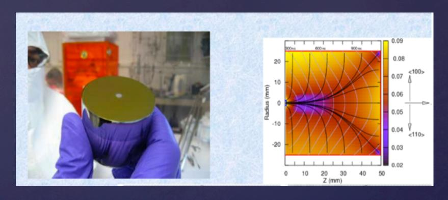
The point contact results in very low capacitance and very low energy thresholds
