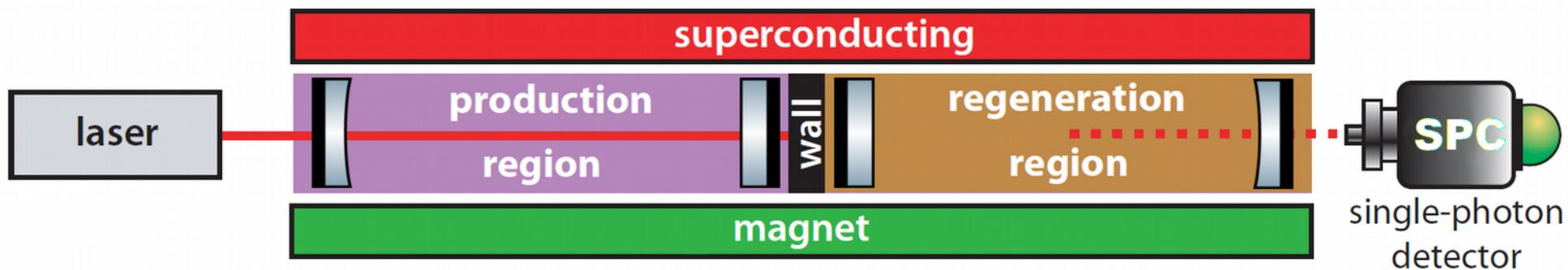
both cavities must be resonant to laser frequency and share same optical axis
