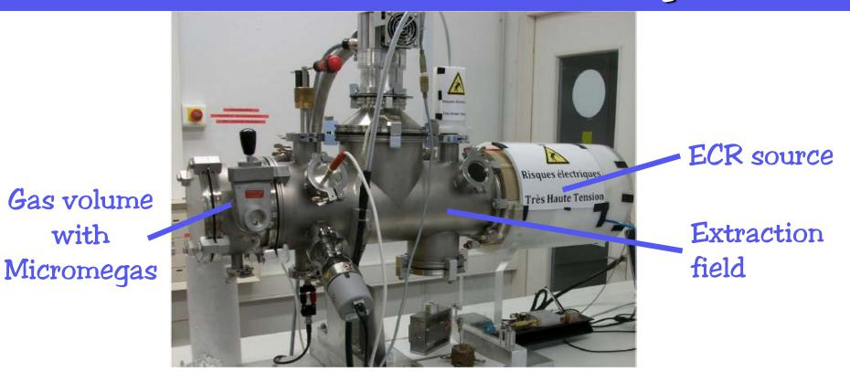
Electron and Ion source from 5 keV to 50 keV being developed at LPSC
